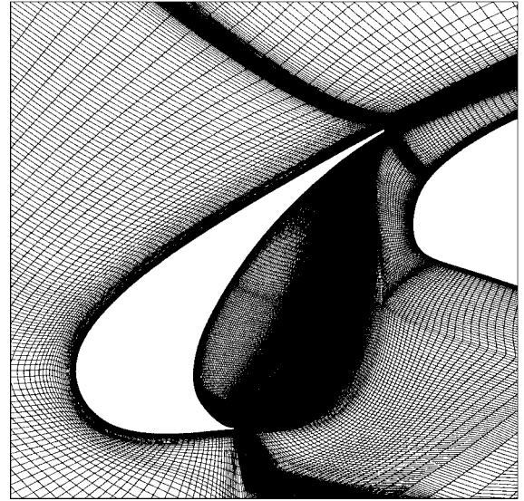
Fig. 17 Fine grid distribution in vicinity of slat; every other point is shown.
